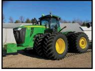
2014 John Deere 9510R 4WD Tractor, 18/6 Powershift Trans, 2081.3 Hrs, 7" GS3 Display, AutoTrac, Premium Cab, 4 SCV, Cat 5 HD Draw Bar, Premium HID Lights, Power Mirrors, Dual Beam Radar Sensor, HD Greasable Steering Pin, Rear Inside & Outside Weight Package, Tool Box, Leather Seating, Instructional Seat, Rock Box, Pre DEF, Firestone 1F 800/70R38s, 2nd Owner, Owners Manual, Receiver Sold Separately, SN-1RW9510RCEP012489
