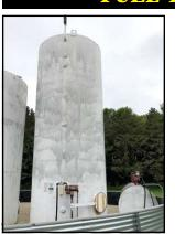
10,000 Gal Vertical Steel Fuel Tank, Used for Clear Fuel, Fillrite pump, Auto Nozzle
