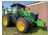
2011 JD 7230R MFWD Tractor, AutoTrac, IVT 40K Trans, LH Rev, TLS Front Axle, Premium Cab, Premium XM Radio, 7" GS3 Touchscreen Display, Foot Throttle, Active Seat, Inst Seat, Power Mirrors, HID Lighting, 1805 Hours Showing, 480/80R46 Rear Duals, 380/85R34 Front Duals, Front Fenders, Radar, (2) 1400# Rear Wheel Weights, 1-3/4" 1000 PTO, 3Pt, Factory QH, 59 GPM Hyd, 5 SCV, Sturd-E-Built HD Rockbox, Bought New, SN-1RW7230RHBD002043
