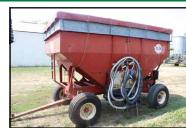
E-Z Flow Model 300 Gravity Box on E-Z Trail 1074 Gear, 12.5L15SL Tires, Ext Pole, with Christainson SV 20 Seed Vac, B&S 10 HP, Elec Start Motor
