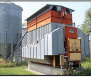
M-C 675EM Continuous Flow Grain Dryer, Small Perforated Screens, Heat Reclaim, Squirrel Cage Fans with (2) 7.5 HP, (1) 10 HP Motors SN- 41915 Wet Holding Bin, (15) Leg Wet Auger, 8"xApprox 30', 5 HP Elec Motor, no transport
