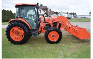
\*\*\* 2018 Kubota M5-111 MFWD, Full Cab With LA1854 Hyd Loader, 83" Bucket, 320/85R24 Fronts, 420/85R34 Rears, 159 Act Hours, 3pt, 2hyd, PTO, Wheel Weights, Joy Stick, Hyd Shuttle Shift, Ultra Grand Cab, SN:56832, **Looks New**
