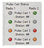
Puller Cart Station: ## - These display the current location, by station number, of the respective puller cart.
