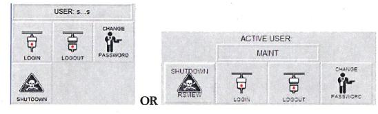
There can be twologin codes: one for Engineering and one for Maintenance. The touch button activates a login and logout screen. A security code is required for authorized personnel. The box above the login and logout touch buttons indicates the active user.
