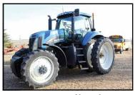
2007 New Holland TG215 MFWD Tractor, SuperSteer, Int. Steering Valve, Fenders, Mirrors, 380/90R54 Rear Duals, 380/80R38 Fronts, (22) Front Suitcase Weights, 4 SCV, PB, 540/1000 PTO, HD Drawbar, Hammerstrap, 3Pt, QH, 2133 Hours Showing, SN-Z6RW04479
