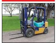
Komatsu 20 LE Forklift, Model FG20C-12, 3230# Lift Cap, 42" Forks, 2 Stage Mast, Pneumatic Tires, LP, 16,378 Hours Showing, SN-51214
